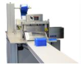
The complete system includes dual unwinds, knife assembly, and shingling conveyor.
